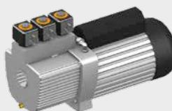
**Vacuum pump with control block** The vacuum pump ensures deep down evacuation of the A/C system. It pumps the evaporated refrigerant into the internal container of the Low Emission service unit, so no refrigerant can escape into the environment.
